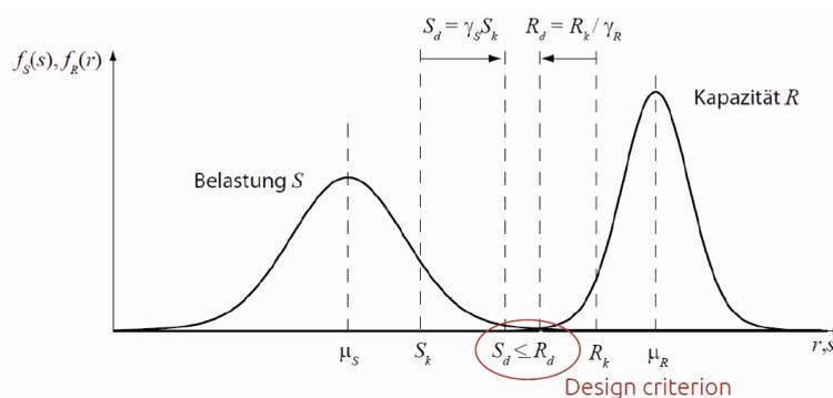
Figure 2: The overlapping region between load (Belastung) and resistance (Kapazität) define situation where the structure will fail [4]
