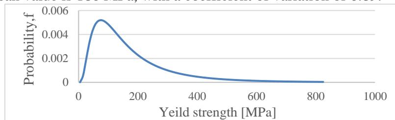
Figure 5: Probability density function, yield strength of reinforcement
