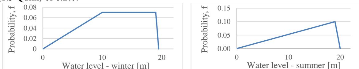
Figure 6: Probability density function for Water level (**Left:** Ice load case - **Right:** Flood case)
