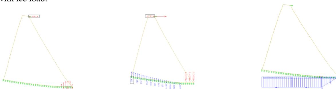
Figure 8: Spring forces (left), deformations (middle) and pore pressure (right) for non-linear analysis. Full pore pressure is assumed in the base area without compression.
